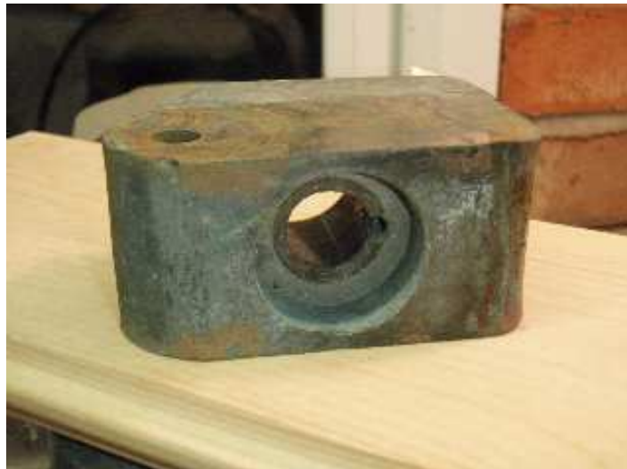
Picture of Rudder Stock showing Keyway
