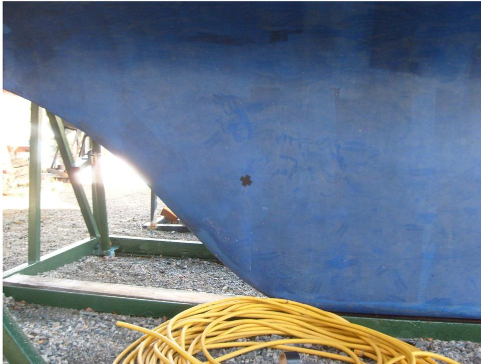
We drilled a 15mm hole and as we got through the GRP we released a foul cocktail that was clearly the cause of the smell. Once this had run out we could see in the bilge where it had got in as the gap was revealed.
